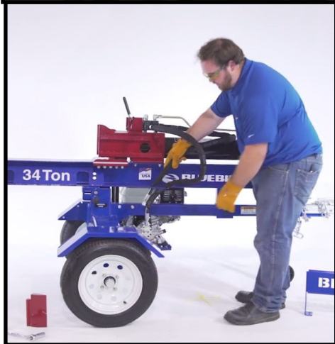
Now route the upper hose down through the inside slot.
