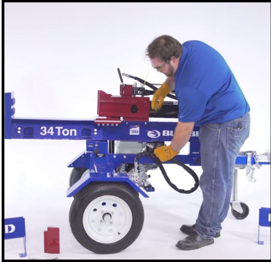
Route the lower hose up through the guide in the outside slot.
