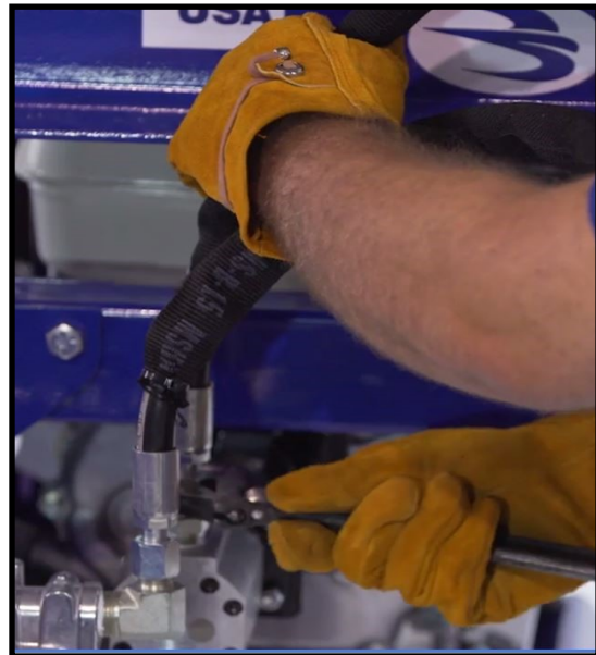
Connect the hose to the pump and tighten all fittings.
